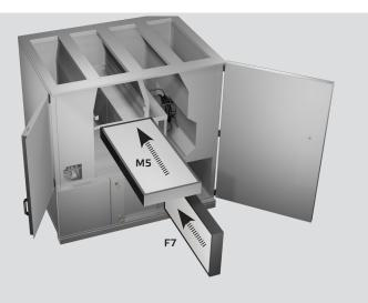
6 Push back the filters clamps, then close and lock the doors.
